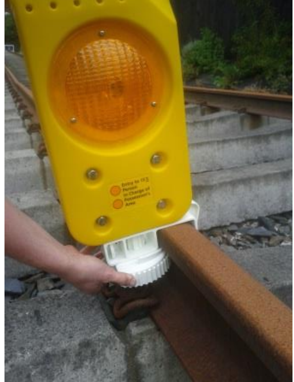
2) Twist cam to lock in place
