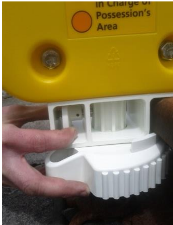
4) Pull release catch to remove from track
