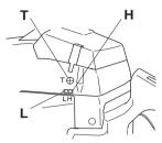
The T-screw regulates the throttle setting at idle speed. If the T-screw is turned clockwise this gives a higher idle speed; turning it anti-clockwise gives a lower idle speed.
