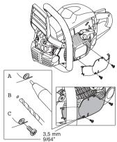
CAUTION! If the special winterising kit has been fitted or any measures have been taken to increase the temperature these changes must be reversed before the machine is used in normal temperature conditions. Otherwise there is a risk of overheating, resulting in severe damage to the engine.
