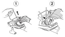
• Undo the screw in the centre of the pulley and remove the pulley. Insert and fasten a new starter cord to the pulley. Wind approx. 3 turns of the starter cord onto the pulley. Connect the pulley to the recoil spring so that the end of the spring engages in the pulley. Fit the screw in the centre of the pulley. Insert the starter cord through the hole in the starter housing and the starter handle. Make a secure knot in the end of the starter cord.
