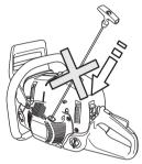
Note! Reactivate the chain brake by pushing the front hand guard back towards the front handle. The chain saw is now ready for use.
