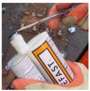
Hold the tubes upright and unscrew the large cap. Carefully prise off the plastic plug in the end of the tube, a small screwdriver is useful for this (you may need this plug later if you only use part of a tube and want to re-seal it).
