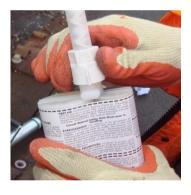
Slide the large cap down over the mixing tube and hand tighten on to the material tubes, ensuring a good seal between them.
