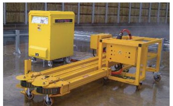
Powervamp extendable cable carrier: options 12–30m (39–98ft), designed for use with all converters and FEGP installations
