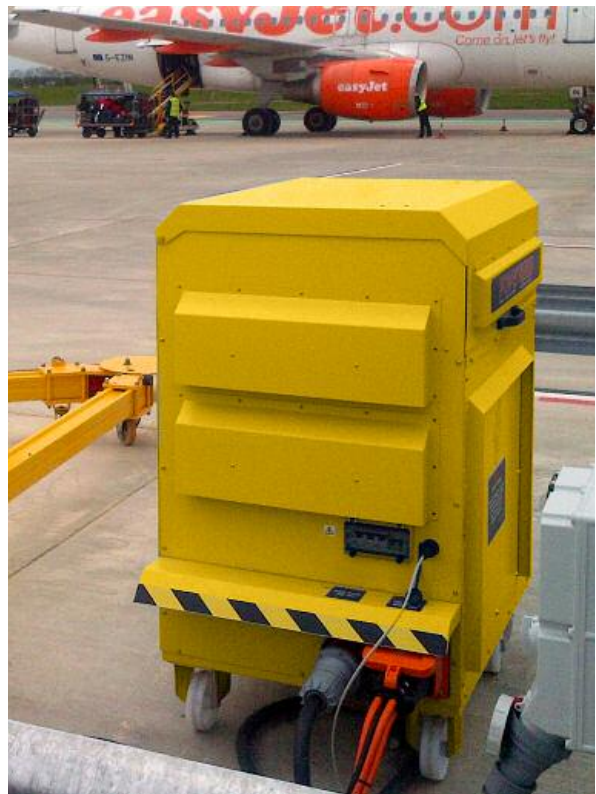
90 kVA showing MABS ethernet connection (see page 26)
