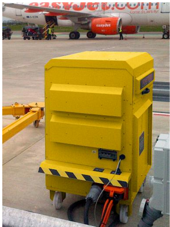
90 kVA showing MABS ethernet connection (see page 26)
