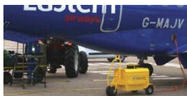
Coolspool 260: First flight of the day, 90 amps for 45 minutes. 1850 amps starting peak
