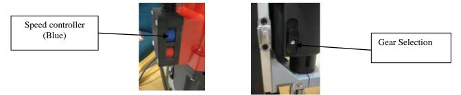
The speed controller is adjusted by rotating the blue disk located on the side of the motor there are 5 speed settings which can be used.
